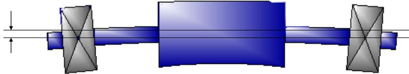
Those tight clearances mean that everything has to be exactly as the designer planned. The whole machine needs to be running precisely as it was designed to be. If the parts are pushed and deformed out of their tolerance, like in this sketch, then the bearings will fail in a matter of hours, and not the years that they should last in a machine that was working as it was designed.
