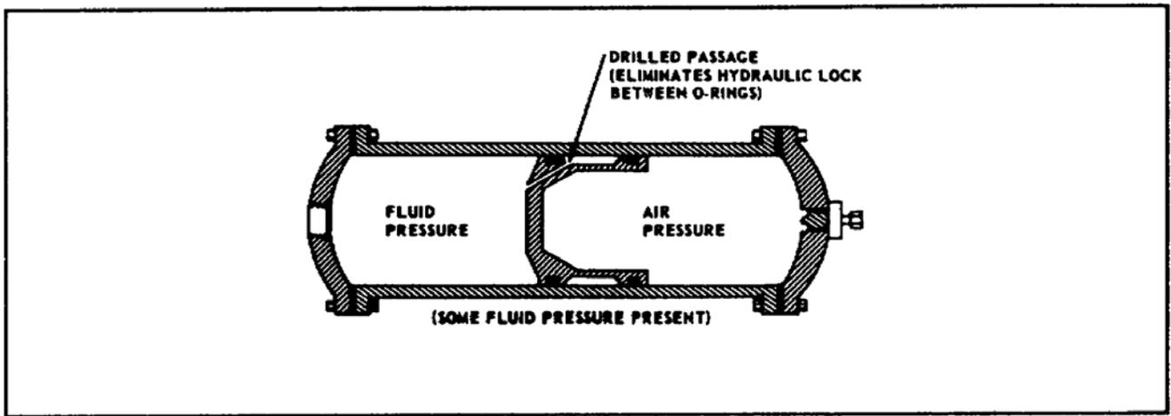
Figure 1-12. Piston Accumulator.
