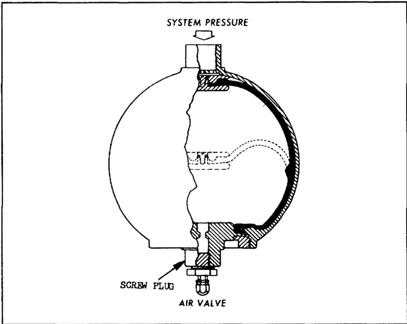
Figure 1-11. Bladder Accumulator.
