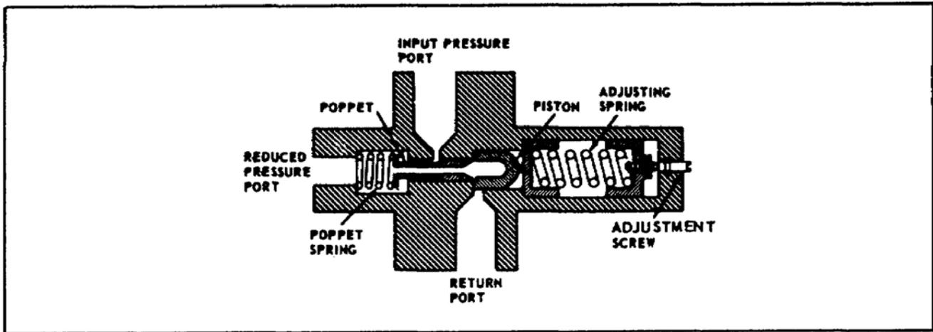
Figure 3-2. Pressure Reducer.
