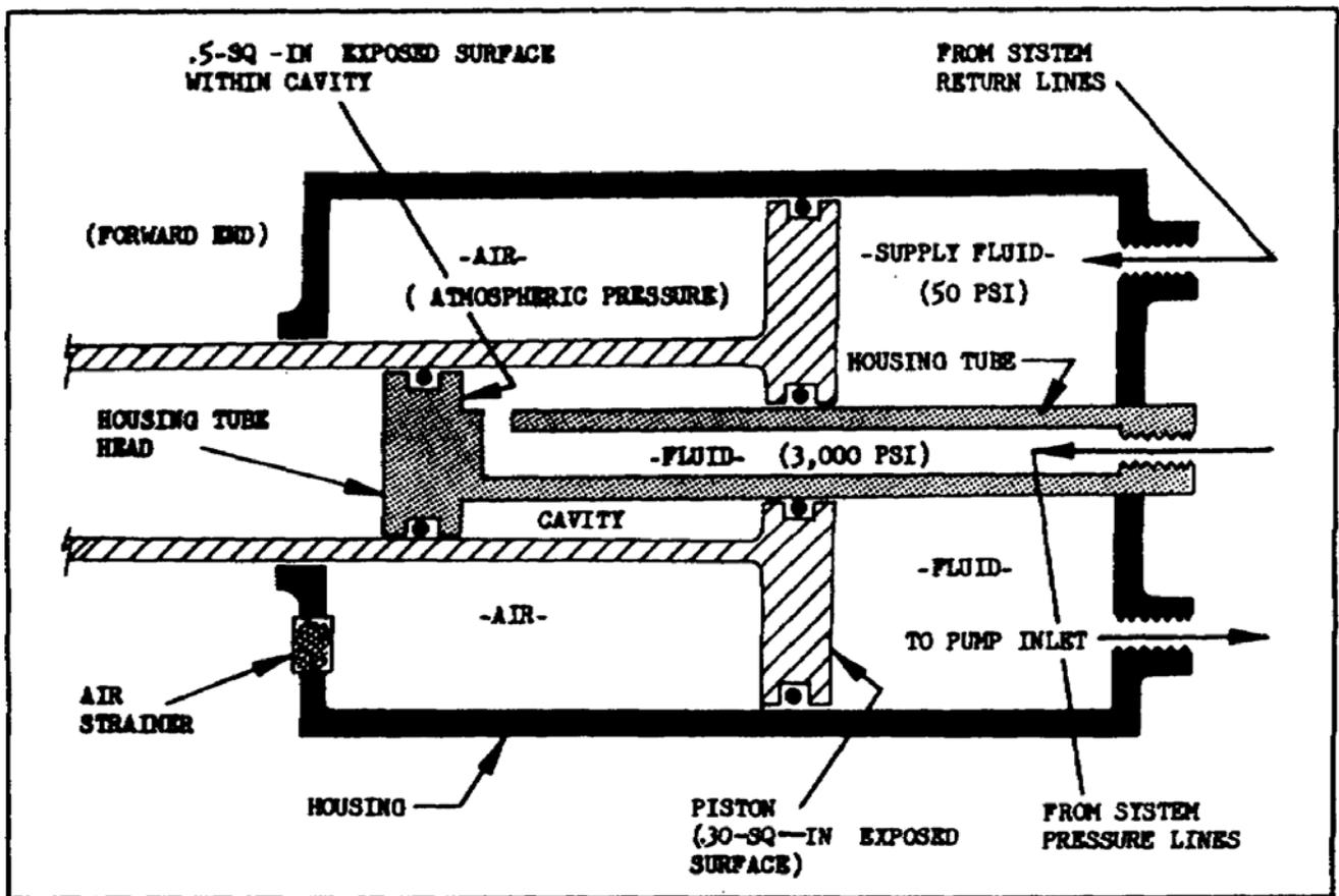
Figure 1-2. Hydraulic Reservoir Pressurized With Hydraulic Fluid.
