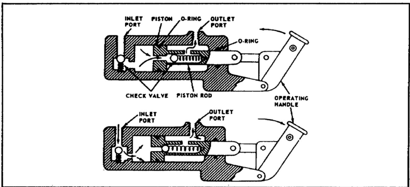
Figure 1-4. Double-Action Hand Pump.
