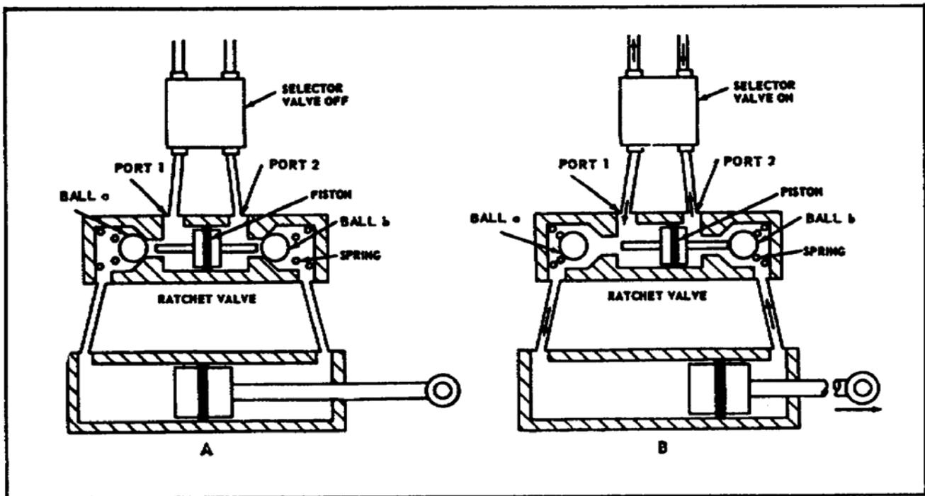
Figure 2-11. Typical Application of Ratchet Valve.
